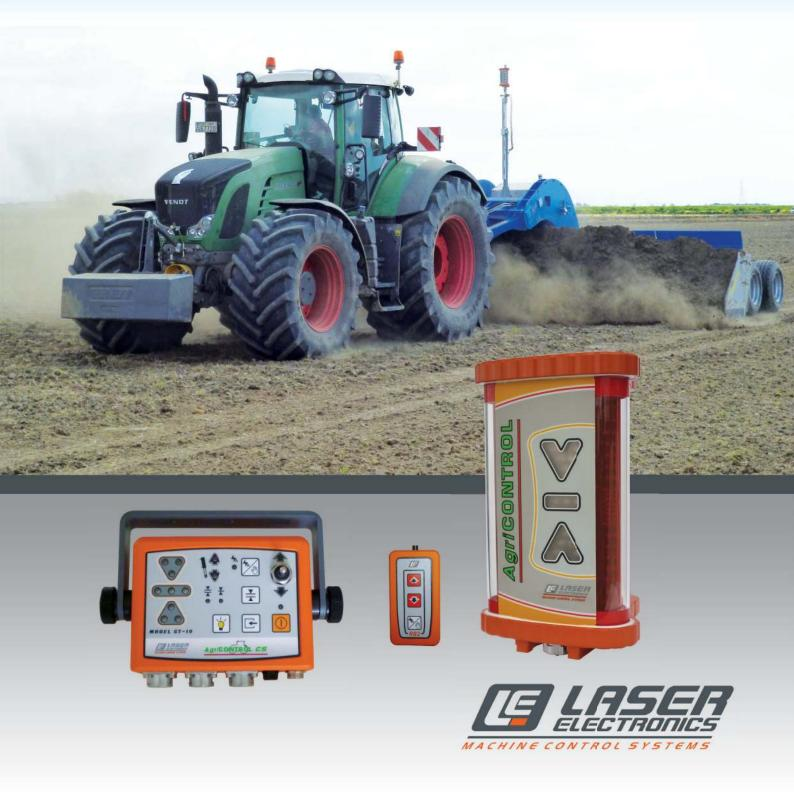
The AgriControl CS is a system for levelling and grading. It can be connected on machines with single cilinder blade control. Applied where level, single or dual grade is required. The system consists of the control unit CT-10, receiver RC-05B, remote (RB2 or RJ-01), the necessary cables and a carrying case.
